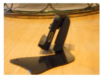
This is the mount with the mount cover installed and a cradle on it sitting on my coffee table. The angle of the mount is about the same as the Garmin mount for the right side.
