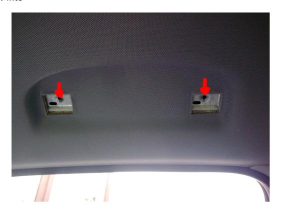
Now the distance inbetween the centres of both hole on the glasses case is shorter than on the BMW handle, (not buy a great deal) so you will need to drill an extra hole to achieve the correct pitch between the holes. You will have to do a bit of measuring to find out were the hole needs to go, but to give you an idea it needs to be roughly here.
