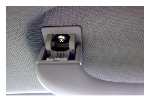
Remove both screws and remove handle. These are the holes the screws screw into
