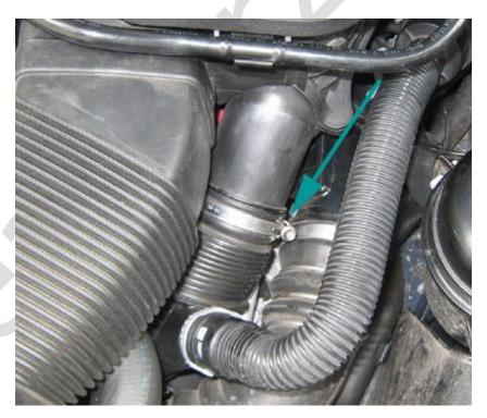
At the back of the airbox is a second hose that is similar. To remove the rear hose, you may need to remove the cable carrier located above the airbox. The cable carrier is secured by 3 clips. To remove the carrier, you will need to push down the lock at the center of each clip and then slide the carrier forward. You will have enough slack in the carrier that you will be able to do them one at a time. In the lower left corner is a close-up of one clip.
