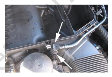
Remove the intake tube by sliding it toward the front of the car. On each side, there is a clip that you need to get over before it will slide. You may need to use a small flat blade screwdriver to get the tube over the clips.
