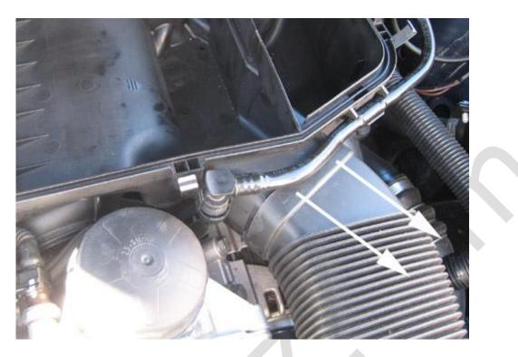
With the larger intake hose disconnected, you can remove the hose located below it. Using a flatblade screwdriver or a 6mm socket, loosen the nut on the hose clamp. You do not need to remove the clamp, it just needs to be loose. Once it is loose, you can slide the hose toward the front of the car and off the airbox.
