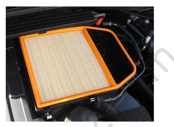
With the air filter removed, you will also want to disconnect the vacuum line at the front of the airbox. To remove it, simply pinch the sides at the base, and lift up.
