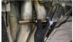
3. Next you will need to unbolt the V flange near the turbo. Keep the hardware as it will be reused (Fig.2)
