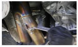
7. Re-Install O2 Sensors before mounting the Vishnu Downpipe for the sake of easy access
