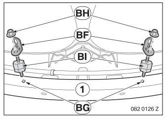
When screwing on rubber bearing **BI**, a suitable screw securing tool must be used. ◀
