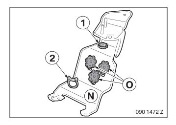
Transfer existing rubber bearing (1) and hose holder (2) of the removed servo oil tank holder to servo oil tank holder  ${\bf N}$ .
