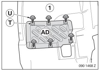
Push sheet metal nuts **T** onto the wheel arch cover (1). Screw on radiator grille **AD** using hexagon sheet metal screws **U**.
