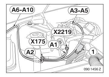
Screw branch **A1** on B+ support point **X2219** from the top or bottom.
