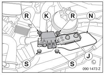
Using the original nuts, screw fan relay holder **J** onto servo oil tank holder **N**.
