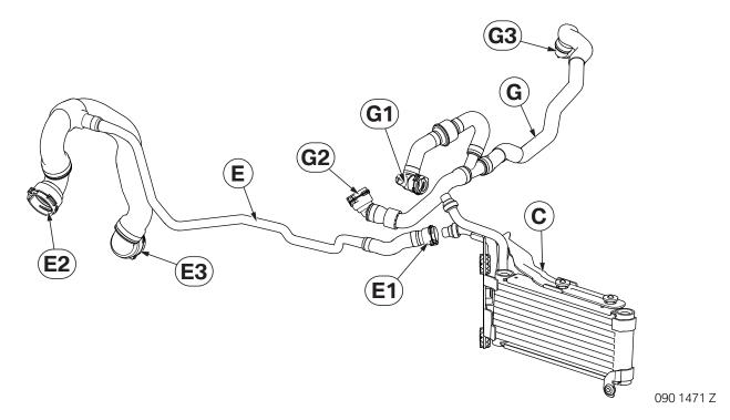
Incorporate return hose **E** and supply hose **G** into the cooling circuit as follows:
