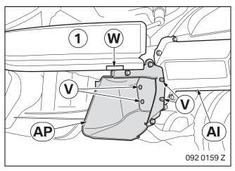
Place front air guide **AP** on rear air guide **AI** and secure from the inside using expanding rivets **V**.
