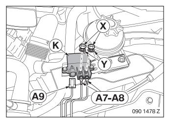
Connect branches **A7–A8** using hexagon nuts **X** and spring circlips **Y** to fan relay **K**.
