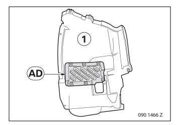
Place radiator grille **AD** from outside onto the wheel arch cover (1).
