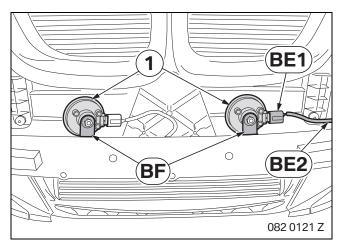
Screw horns (1) using original nuts and washers to retaining bracket **BF**.
