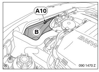
Install electric fan **B** (see ISTA 17 11 035) and connect branch **A10**.
