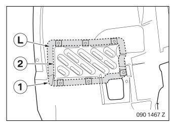
Mark the cut-out (1) 20 mm inside contour (2) of radiator grille  ${\bf L}$  and cut out.
