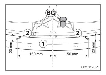
Make drill holes (2), diameter 9.1 mm, from above on the bumper support (1) as per the dimensions shown.
