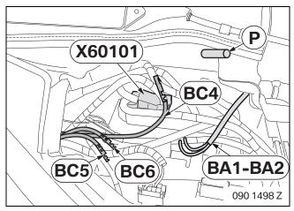
Push shrink tubing **P** over branches **BC5**, RT/GN cable, and **BC6**, BR cable.
