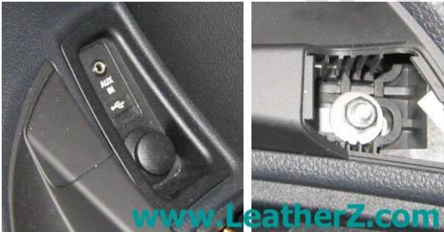
Remove the 10mm nut (make sure you do not drop the nut into the center console). Set the cover and the nut off to the side.
