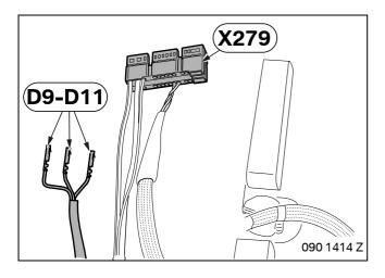
Connect branches **D9–D11** as follows to the seat isolator plug on the passenger side, GE 19-pin socket casing **X279**:
