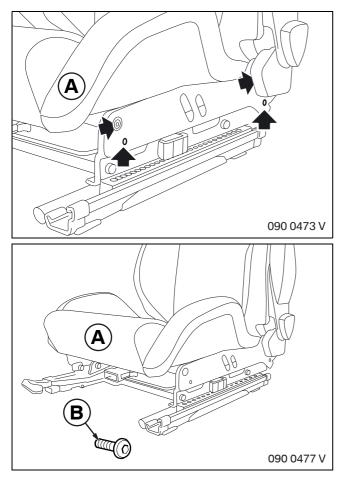
BMW Performance sport seat **A** can be installed at a height to suit the individual customer using the holes (arrows).
