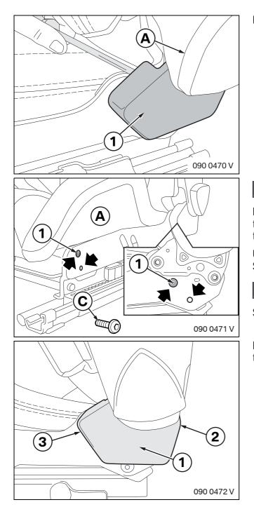
Remove cover cap (1) from sport seat **A** using a suitable tool.
