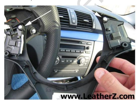
With the screws holding the controls in place removed, you can remove the trim completely.
