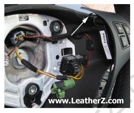
The wiring for the steering wheel controls is still connected so be careful removing the trim. There is enough slack to access the back of the trim. To remove the steering wheel controls, remove the T-20 screw at the top location.
