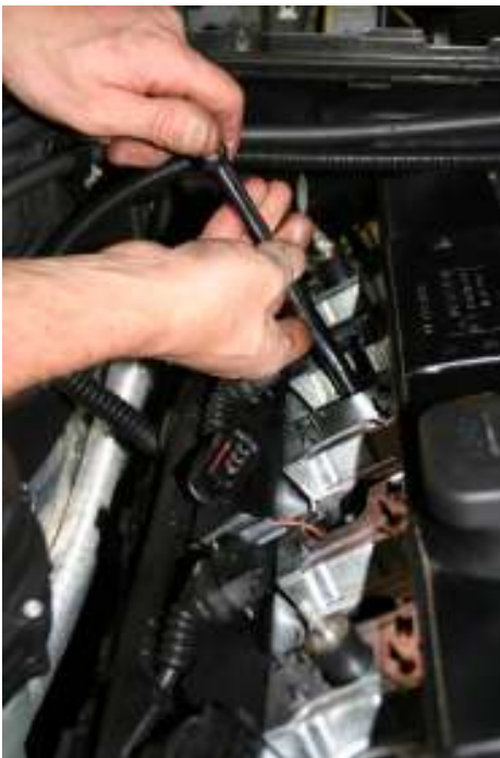
Replacing spark plugs in an M54 engine.
