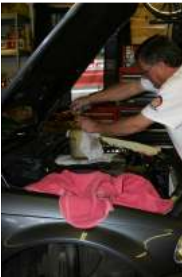
BMW Master Technician John Franchetti hooks up a pressure bleeder during a brake fluid change on a supercharged E46 330Ci convertible.
