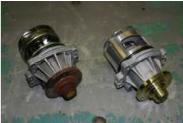
OE/OEM water pump (l), compared with EMP Stewart High Performance Water Pump. The pump on the left has a metallic Impeller – that doesn't make any difference in longevity. Both the plastic and metallic impeller OE/OEM pumps fail prematurely, just in different ways.
