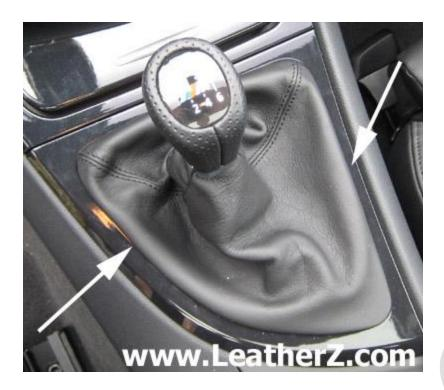
With the Shift Boot undocked, remove the shift knob. The shift knob lifts straight up off the shift lever. Do not turn or twist it. Just pull straight up. Some shift knob can be stubborn so be careful, plenty of BMW owners have hit themselves in the face when the shift knob finally lets go.
