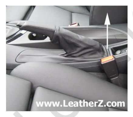
With the Boot unclipped, slide the boot forward over the brake lever. You will turn the boot inside out as you go.
