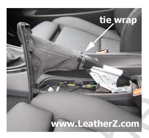
At the base of the Emergency Brake Handle is a tie wrap that secures the boot. Cut the tie wrap and the boot will able to come off.
