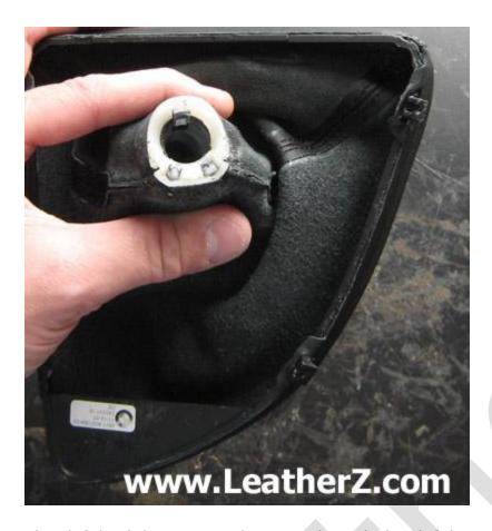
The shift knob has 3 teets that pass through the shift boot and lock into the disc. To remove the disc, use a small screw driver and carefully pry it off. Go slow and be careful.
