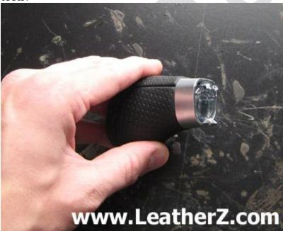
If you are switching to an aftermarket shift boot and want to use your stock shift knob, you will need to remove the teets from the bottom of the shift knob. Carefully cut them off with some wire snips
