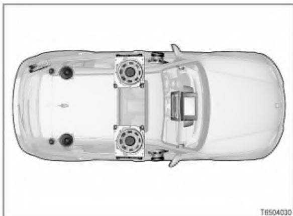
6 channels (7 channels simulated - Logic7)
