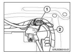
1. With the ignition turned off and any external power source removed, access the HV interlock loop safety connector by removing the trunk floor panel. The safety connector (1: shown in its normally locked position) is located near the 12V vehicle battery's ground terminal (2).
