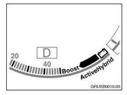
Hard acceleration will briefly utilize the electric motor for boost function.
