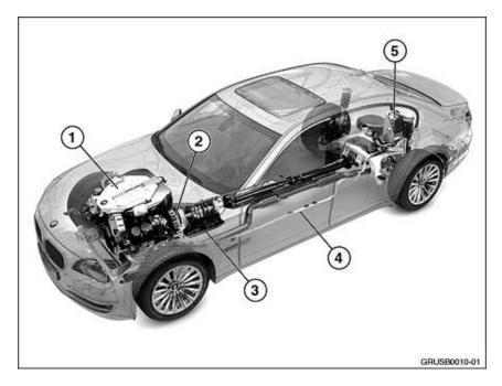
1 N63 engine 2 Electric motor 3 Transmission 4 HV lines 5 HV battery pack
