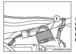
3. Secure the safety connector from being inadvertently reconnected while repairs are still being performed by using a conventional padlock (1). The technician must keep the key on his person during repairs.
