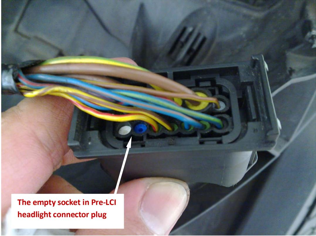
**The empty socket in Pre-LCI headlight connector plug**
