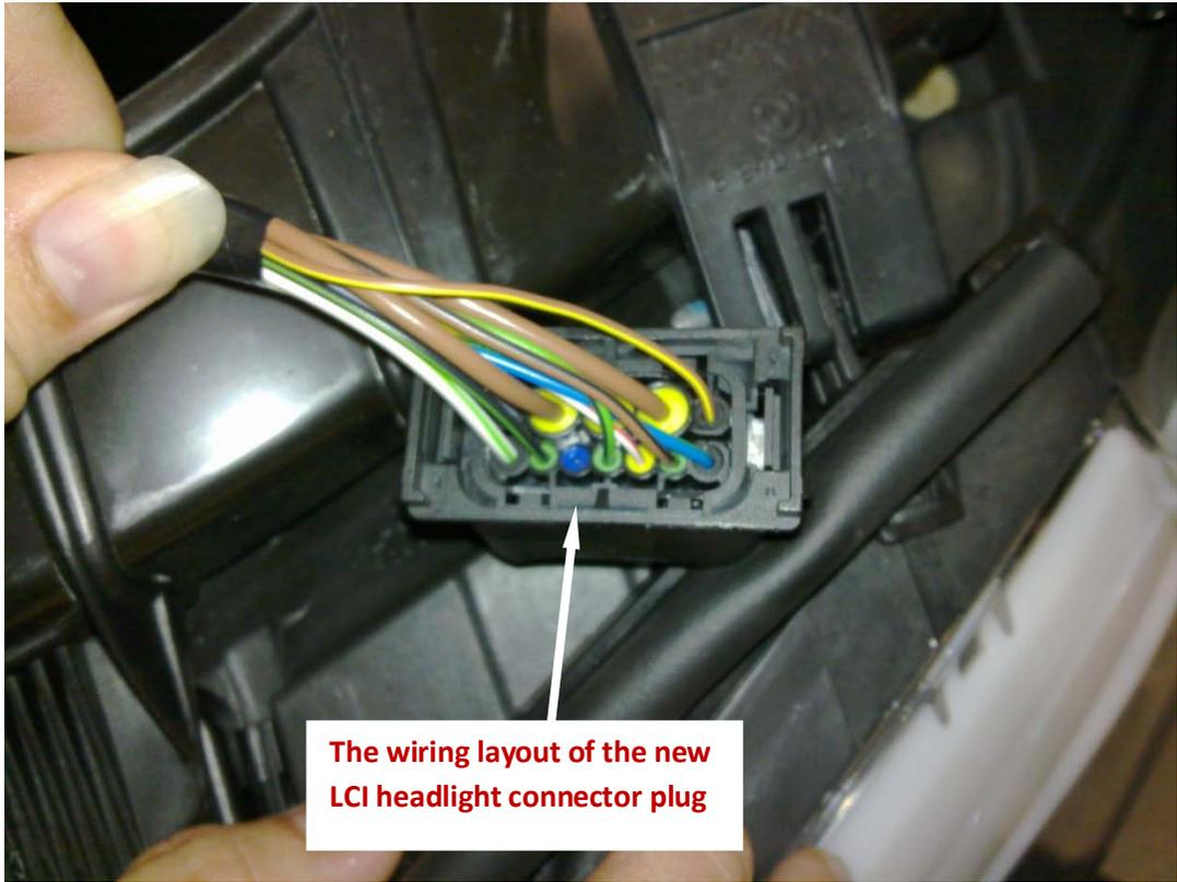
**The wiring layout of the new LCI headlight connector plug**
