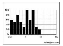
A history of the energy flow is available in the CID, found by selecting "Vehicle Info", "Hybrid", then "Hybrid Usage". The display is updated every minute and shows the percentage of driving time during which the hybrid system provided either driving support or energy recovery during the last 15 minutes.
