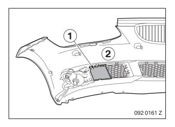
**E92/E93 automobiles with M bumper only** Unclip left cover (1) behind grille from bumper (2) (it is no longer needed).
