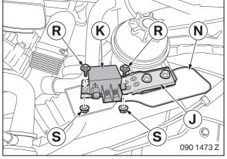
Transfer existing rubber bearing (1) and hose holder (2) of the removed servo oil tank holder to servo oil tank holder  $\mathbf{N}$ .
