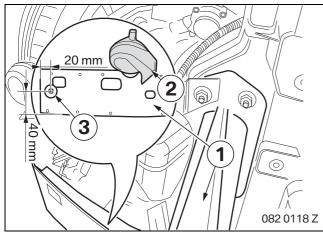
Make a drill hole (3), diameter 8.5 mm, on the bumper support (1) as per the dimensions shown.
