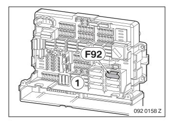
Remove fuse **F92** from front fuse holder (1) (it is no longer needed).
