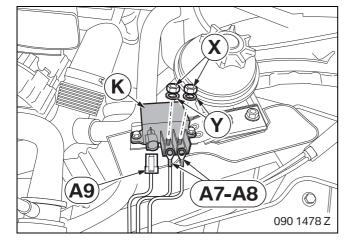
Connect branches **A7** – **A8** using hexagon nuts **X** and spring circlips **Y** to fan relay **K**.
