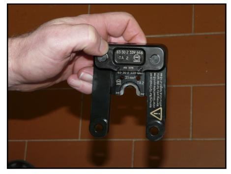
20. Insert the upper die into the tool (as shown) until it locks in place.
