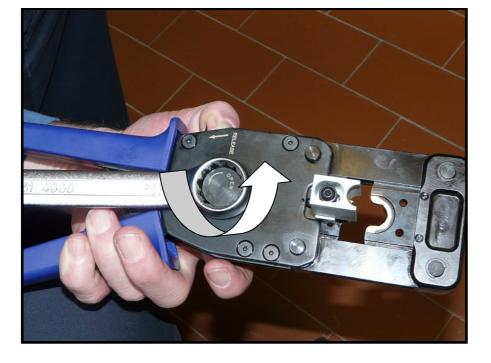
22. Using the wrench supplied with the tool, open the tool by holding the release lever and turning the nut counterclockwise.
