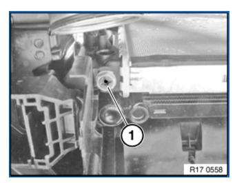
Open coolant drain plug (1).
