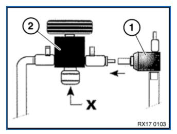
Connect Venturi nozzle (1) to vacuum filling unit (2). (X) Expansion tank connection
