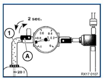
Then open shutoff valve (A) until the filling hose (1) is free of bubbles.
