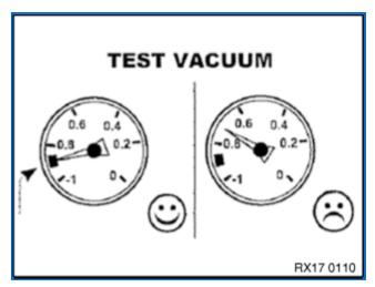
The cooling system must hold the vacuum for 30 s. If the needle in the pressure gauge drops, this indicates a leak in the cooling system.
