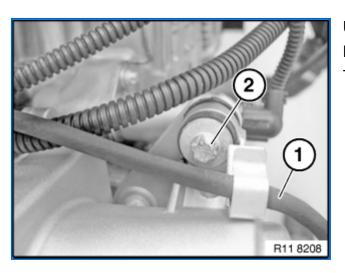
Unclip cable (1) from bracket. Release screw (2). Tightening torque 11 51 2AZ.
