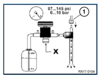
Connect compressed air (1). (X) Expansion tank connection
