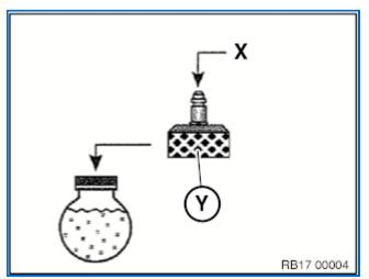
Select adapter (Y) according to table and connect to coolant expansion tank.
