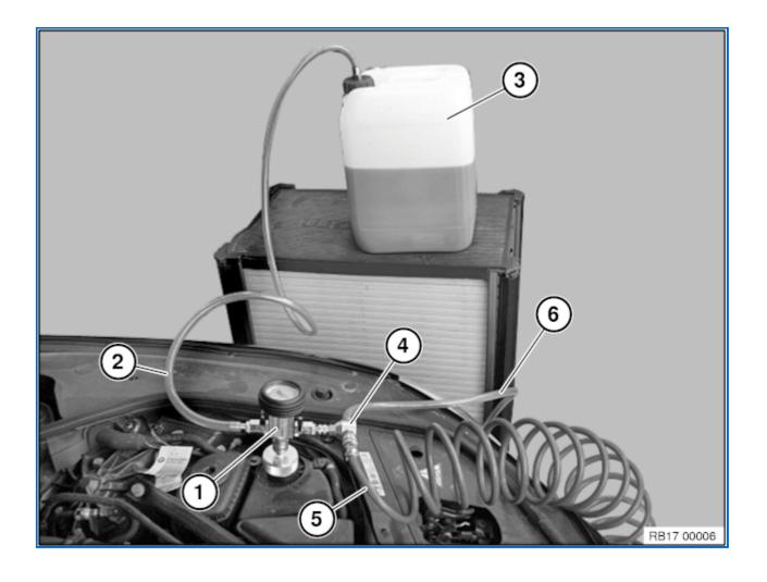
• 1) Vacuum filler device with pressure gauge and shutoff valves
