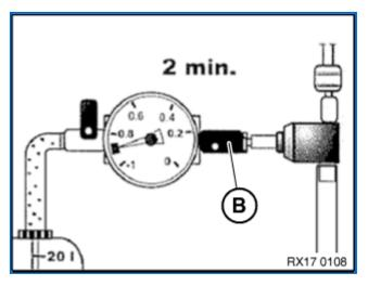
Shutoff valve (B) will remain open. Generate vacuum in coolant system for approx. 2 minutes. The final vacuum is reached at a vacuum of -0.7 to -0.95 bar. Green scale in the pressure gauge.
