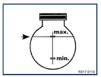
Adjust coolant level to maximum. Close coolant expansion tank.
