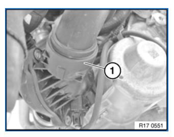
Unfasten and detach coolant hose (1) from thermostat housing.
