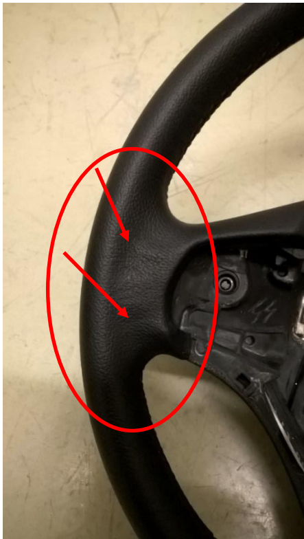
Not OK example - Leather steering wheel (base version) – blistering visible at the steering wheel clasp → covered by warranty
