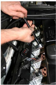
Replacing spark plugs in an M54 engine.
