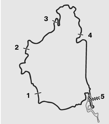
The SECTION race timer enables individual laps to be divided up into sections (max. 9 sections). The values travelled (times, speeds, acceleration forces) are stored and can be displayed later. The example shows a measurement on the Nürburgring (north loop) with 5 sections (see figure).
