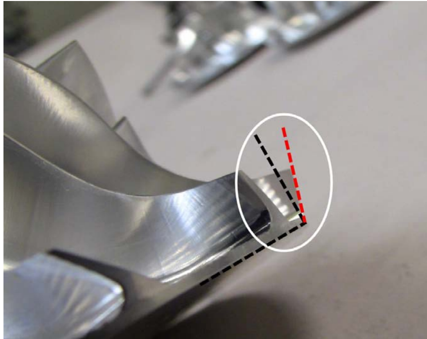
Figure 42: Extended Tip Technology (ETT) on EFR and Airwerks Product Lines
