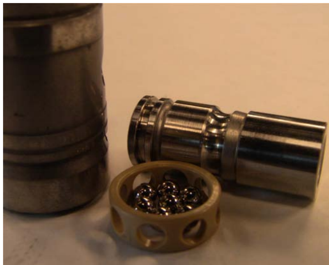
Figure 27: Competitor's Plastic Cage and Steel Balls
