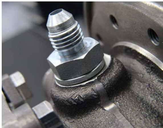
Figure 30: -4AN Oil Inlet Fitting (Supplied)
