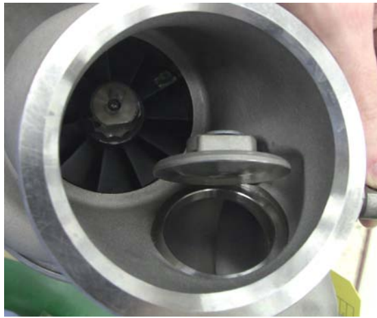
Figure 16: Large Internal Wastegate
