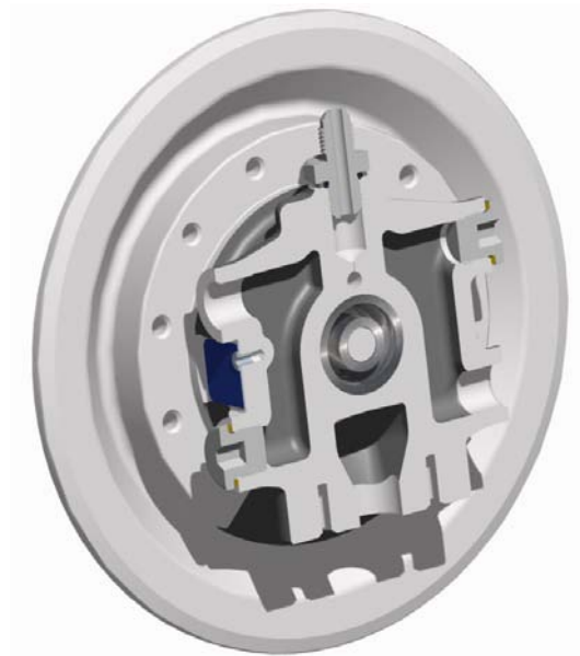
Figure 102: Oil and Water Cavity Detail
