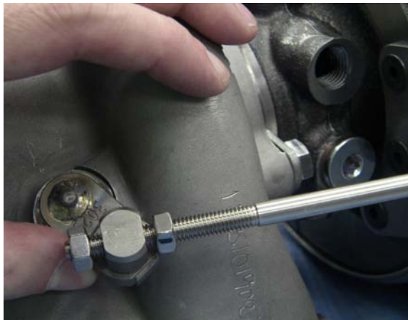
Figure 83: Holding Valve Closed with Nuts Loosened
