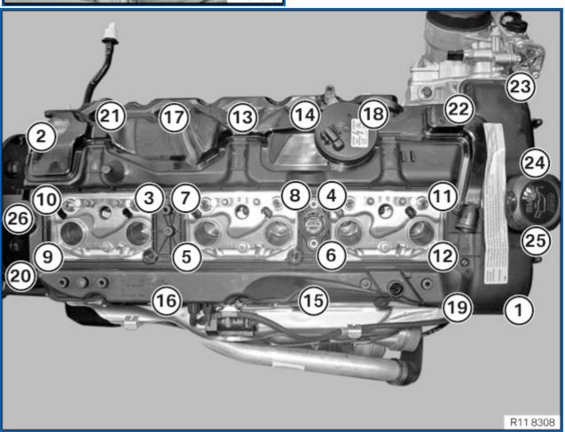
Loosen screws of cylinder head cover from outside inwards in 1/2 turns. Remove cylinder head cover.
