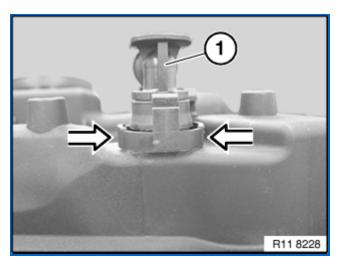
Press and hold down the unlocking device on the vacuum line (1) on the vacuum reservoir (cylinder head cover) in the direction of the arrow.
