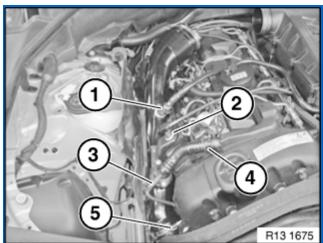
Do not loosen the engine vent line (4) on the cylinder head cover.
