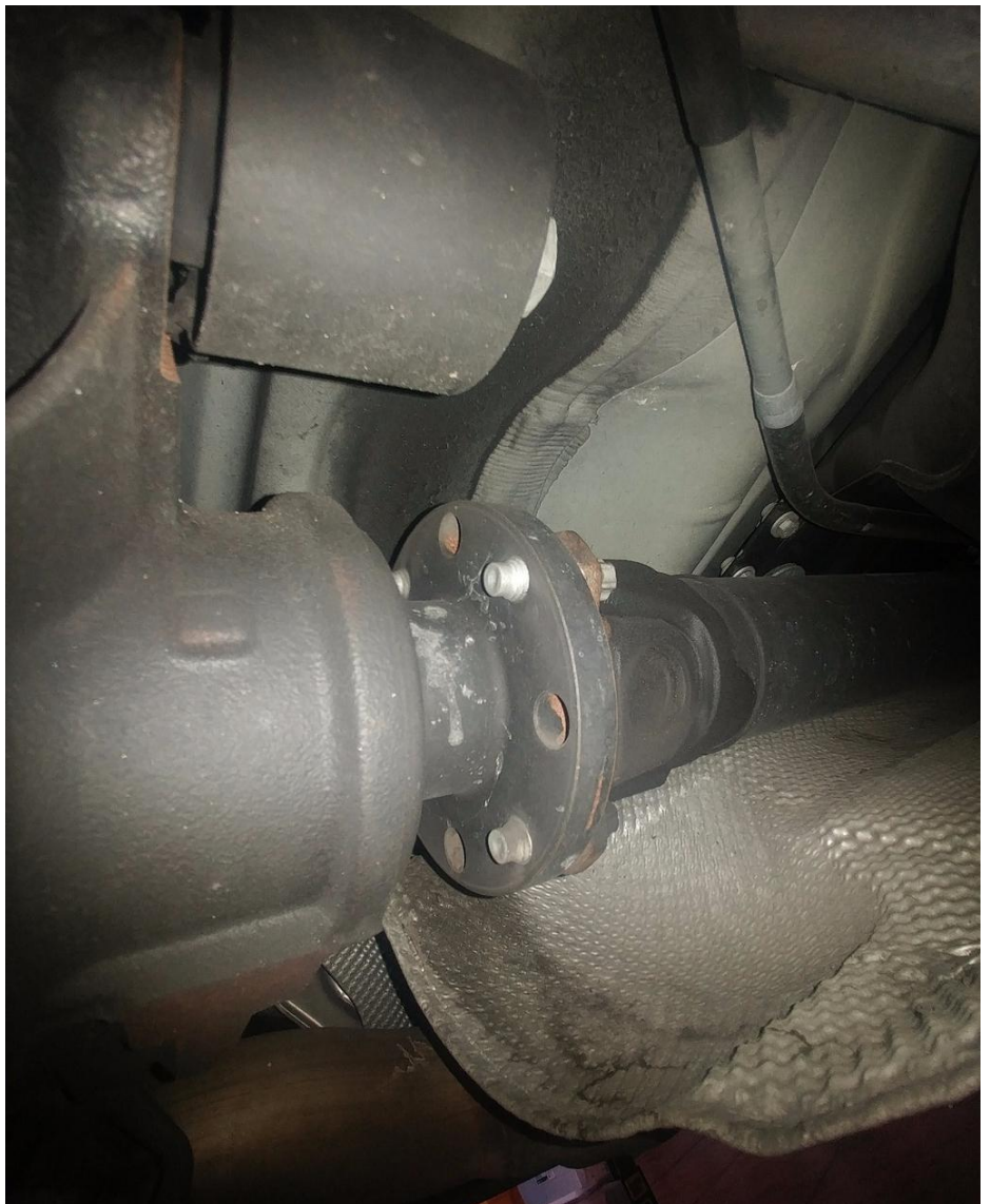
Remove the 10mm bolt and bend the heatshield away from the driveshaft. Remove the E12 bolts. Grab a friend to sit in the car operating the e-brake so you can break a bolt loose, turn the shaft, then break another bolt loose.
