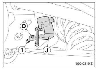
Place the rear holder **J** in the hole (1) and secure it with a hexagonal screw **O**. Tightening torque 8 Nm.
