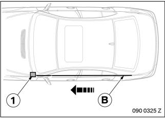
Route the rear level sensor wiring harness **B** along the standard wiring harness into the footwell on the driver's side (1).
