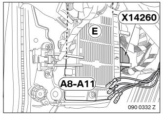
Connect branches **A8 - A11** as follows to plug **X14260** (51-pin SW) in the footwell module **E**:
