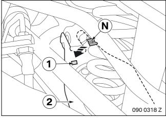
Position the expanding nut **N** in the opening (1) on the left camber control arm (2).
