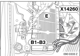
Connect branches **B1 - B3** as follows to plug **X14260** (51-pin SW) in the footwell module **E**:
