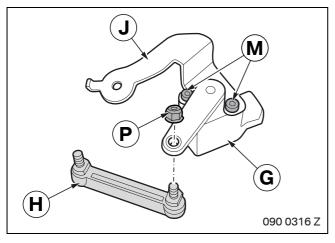
Secure the level sensor **G** as shown to the rear holder **J** using Allen screws **M**. Tightening torque 5 Nm.
