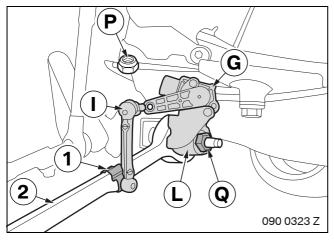
Secure the front holder **L** with collar nut **Q**. Tightening torque 68 Nm (see TIS RA 31 12 000).
