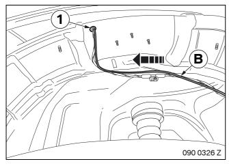
Route the rear level sensor wiring harness **B** along the ABS sensor cable and through the grommet (1) into the interior.
