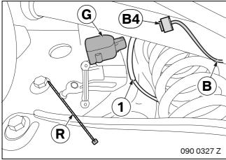
Connect branch **B4** to level sensor **G**.
