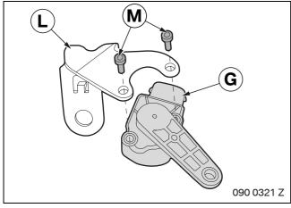
Secure the level sensor **G** to the front holder **L** using Allen screws **M**. Tightening torque 5 Nm.
