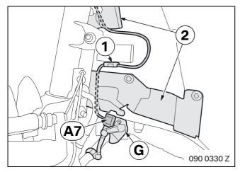
Route branch **A7** (6-pin BR plug) along the standard wiring harness to the front level sensor **G** and connect it.
