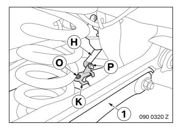
Secure the control rod holder **K** to the camber control arm (1) using a hexagonal screw **O**. Tightening torque 8 Nm.
