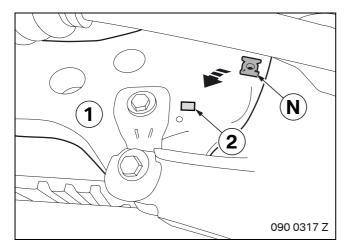
Position the expanding nut **N** in the opening (2) on the front of the left axle mounting (1).
