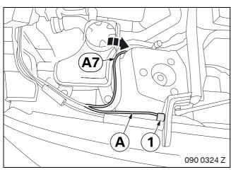
Route branch **A7** (6-pin BR plug) along the standard wiring harness into the wheel arch.
