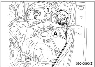
Thread the wiring harness **A** through the grommet (1) into the interior.
