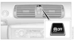
Push the button: the indicator lamps for MDM and DSC OFF light up.
