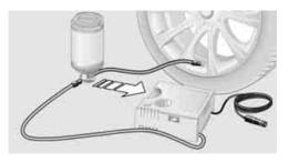
5. Screw the filler hose of the sealant bottle onto the valve of the faulty tire.
