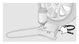
8. With the ignition switched on or the engine running, switch on the compressor.
