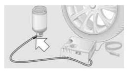
Insert the sealant bottle into the housing of the compressor so that the bottle is upright.
