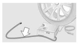
Screw the connecting hose to the connection of the sealant bottle. Do not kink the hose.
