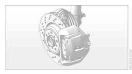
Your BMW 1-Series M Coupe is equipped with a high-performance brake system with perforated compound brake discs.
