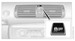
Press the button for at least 3 seconds until the indicator lamp for DSC OFF lights up and DSC OFF is displayed in the instrument cluster. DSC and M Dynamic Mode are both deactivated. Stabilizing and drive-output promoting actions are no longer executed.
